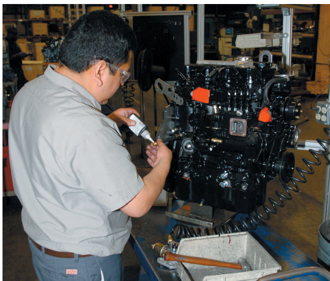
Top: Diesel engines as they arrive from several manufacturers, awaiting conversion to become Westerbeke products with the use of additional components from around the world. Above: Westerbeke parts go onto the engine in a subsequent station in the assembly. This worker will also check the work done by the previous station and keep track of any issues or problems found. This quality assurance process works well. Inset: Pumps and other essential parts are stored in bins for use in the assembly process. The company's just-in-time philosophy means that there are dozens, not thousands, of such parts kept in the Taunton facility.
