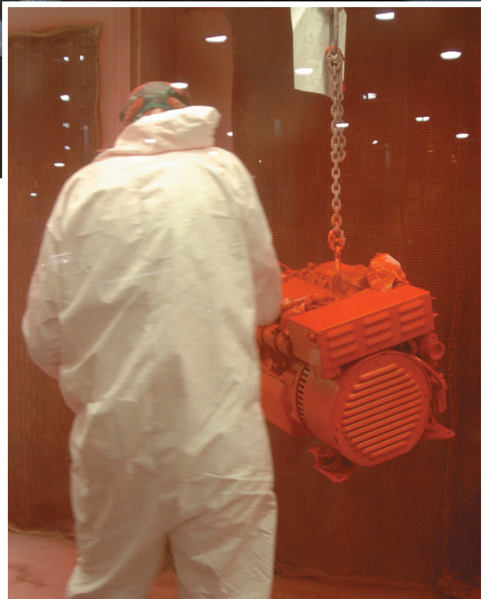
Top: Coming out of the baking oven that cures the paint, every engine and generator receives its various labels, model plates, and other tags. Above left: Bolted to a pallet, another new Westerbeke unit is readied for shipping worldwide. Above right: Inside the elaborate and high-tech paint shop, a generator is painted in the familiar bright red that has become Westerbeke's signature.
