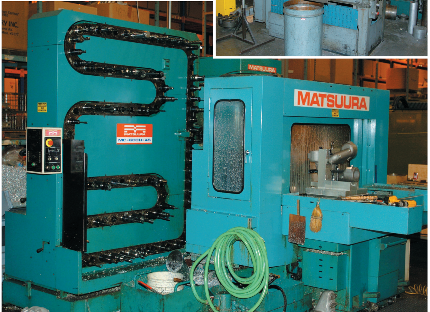
Top: Old conventional manufacturing equipment still has a productive life at Westerbeke, and employees have the craftsmanship to use it on a regular, if not frequent, basis. This is a band saw from the early 1900s. Above: The latest computer-controlled drilling, shaping, and other tooling equipment allows for precise and consistent production of custom parts for the Westerbeke line.
